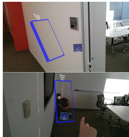
Figure 3: Examples of object detection results sent via canine and seen by handler wearing HoloLens-2.
